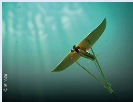
Kite surfing in tidal current: The seven ton power station proves to be very efficient in practice.
